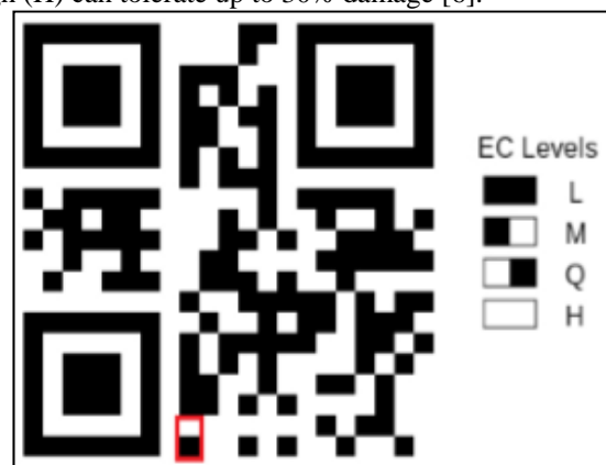
Fig. 3: Error correction level of QR Code[4]
